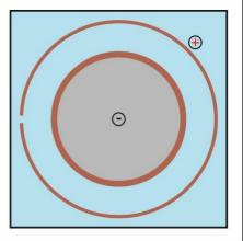
If the shape is adapted to the workpiece, the metal is deposited much more evenly. The layer is thinner on the side facing away from the anode. Overall, the layer is much more uniform compared to a flat anode.
