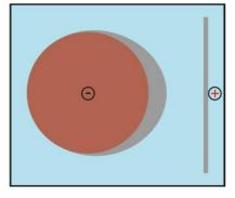
Good scattering (e.g. copper acid) when using a flat anode. The smaller the distance, the more current flows at these points and more metal is deposited there. Due to the good scattering, a thin layer is still deposited on the back.
