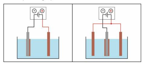
The anode and the workpiece are positioned opposite each other. More metal is deposited on the front side of the workpiece than on the rear side. The workpiece should be rotated at regular intervals.
